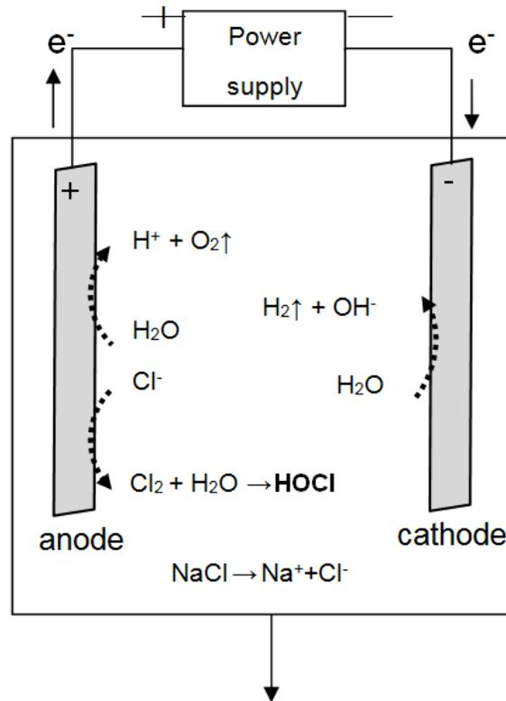
**Fig. (2):** The schematic diagram of hand-made membrane-less electrolyzing device. (Hsu *et al.*, 2019).
