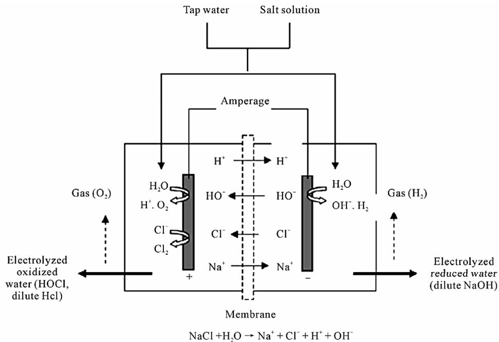
**Fig.(1):** Schematic diagram of EO water generation system (Subrota *et al.*, 2012).
